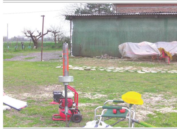
FIG. 7: INDAGINE SISMICA (SN) E PROVA PENETROMETRICA (DX)
